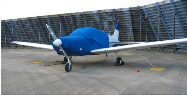
b) If parked outside, use control locks and proper tie-downs to guard against winter gales. Face into the prevailing or forecast wind. Unlike the picture, put proper pitot and static covers on – make sure the pitot has cooled down!
